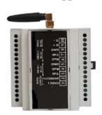
The IoT gateway is a Microcontroller based product with GSM interface for connecting field instruments with cloud. It collects real time data from field instruments and pushes data to cloud server. Data stored at cloud server can be viewed from remote places. The gateway stores data in local non-volatile flash memory in case of network issue and sends data to the server when network connection is restored to avoid data loss. It supports MQTT Protocol.
